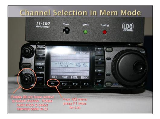
Hold MENU/GRP button 1 second to toggle between memory groups M, S, G(graphics) Select M-2 Press F-4 for V/M Press F-1 (MEM, LST) twice to enter memory channel List Push (PBT/M-ch/RIT) knob to enter (M-ch/RIT) function Rotate (M-ch) inner control to select channel. Rotate outer knob to select memory bank (A-E) Exit memory channel press MENU/GRP
