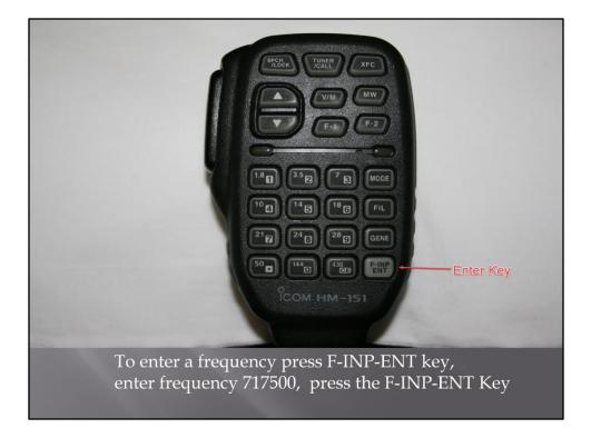
Most functions can be control from the microphone.
