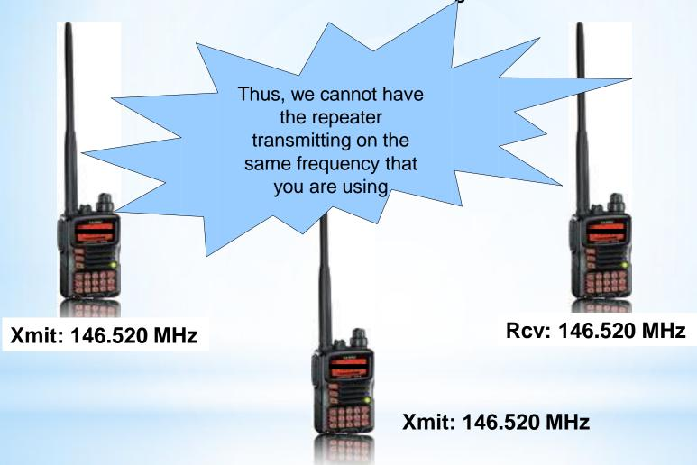
The sender (you) and the repeater each have to transmit on a different frequency
